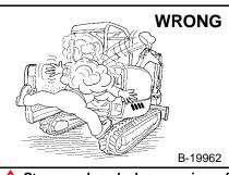
A Stop, cool and clean engine of flammable materials before checking fluids.
