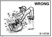
Lead-acid batteries produce flammable and explosive gases.
